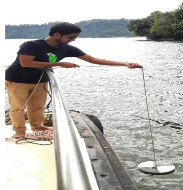
Figure 04: Determination of transparency
