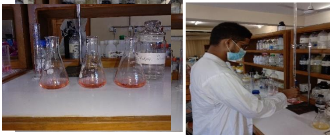
Figure 07: Determination of Alkalinity
