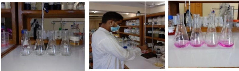
Figure 08: Determination of CO 2
