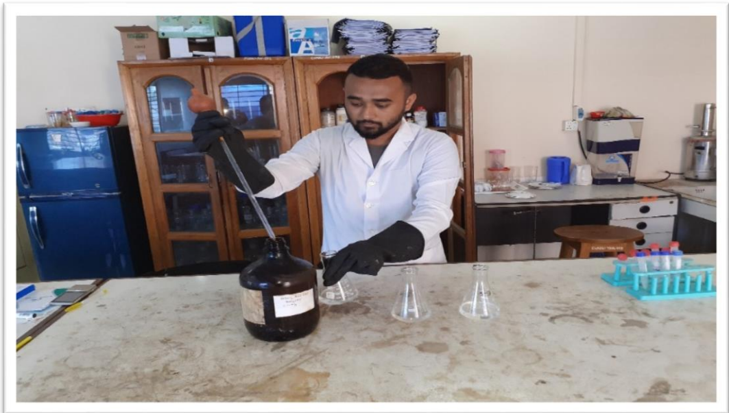
Figure: Addition of \text{H}_2\text{SO}_4 into filtrated water
