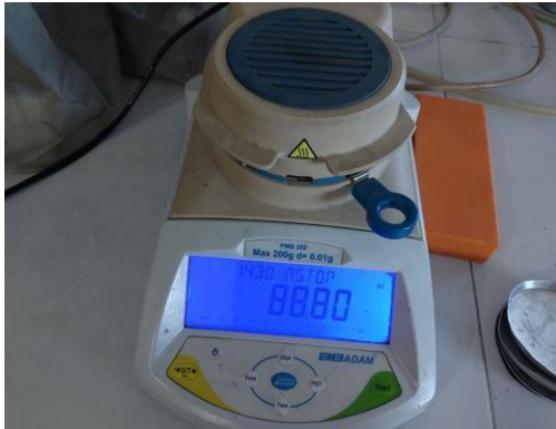
Figure 1: Measurement of Moisture
