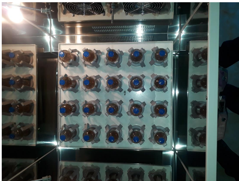
Fig.2.1: Serum bottles with feed sample and buffered Rumen fluid in shaking incubator
