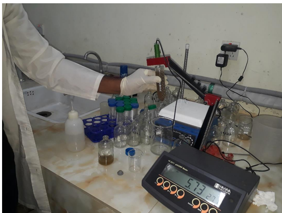
Figure.2.3: After digestion pH measuring with pH meter
