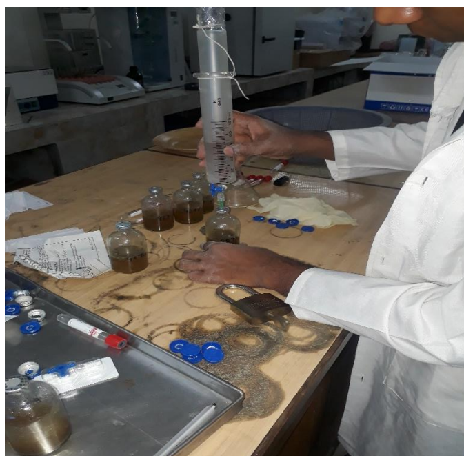
Fig.2.2: Collection of Total gas from serum bottles
