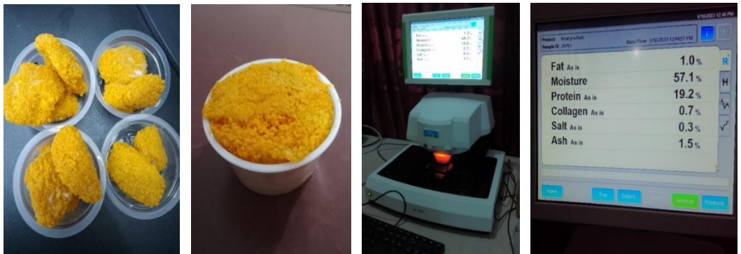
Proximate analysis (nutritional evaluation) of products by using Perkin Elmer NIR machine
