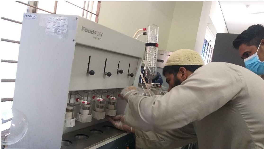
Plate 15: Proximate composition analysis of prepared feed
