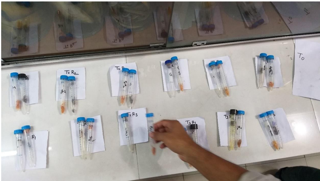
Plate 18: Take 1 g fish sample in test tube
