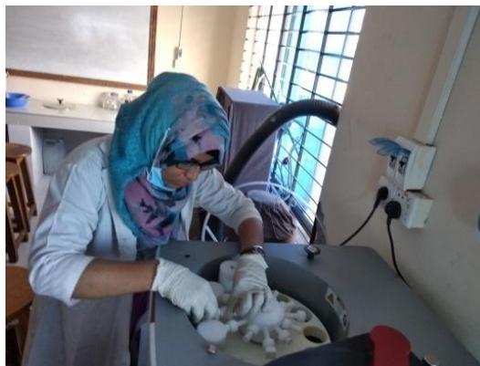
Plate -18: Set up tube for microwave digestion Plate -19: Sample taken into test tube
