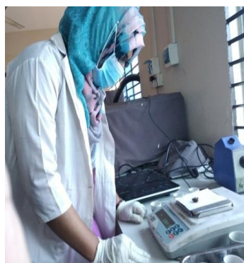
Plate -15: Weighing of dried sample
