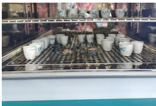
Plate -13: Drying in hot air oven
