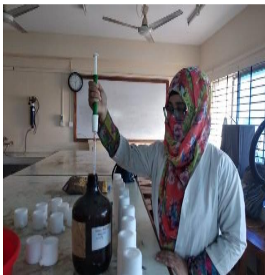
Plate 12: Acid mixing for digestion
