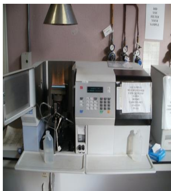
Plate 15: Atomic Absorption Spectrometry for metal analysis
