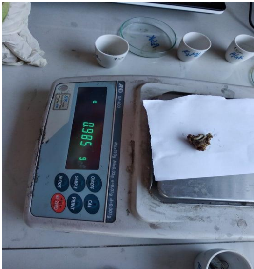
Plate10: Sample weighing for drying
